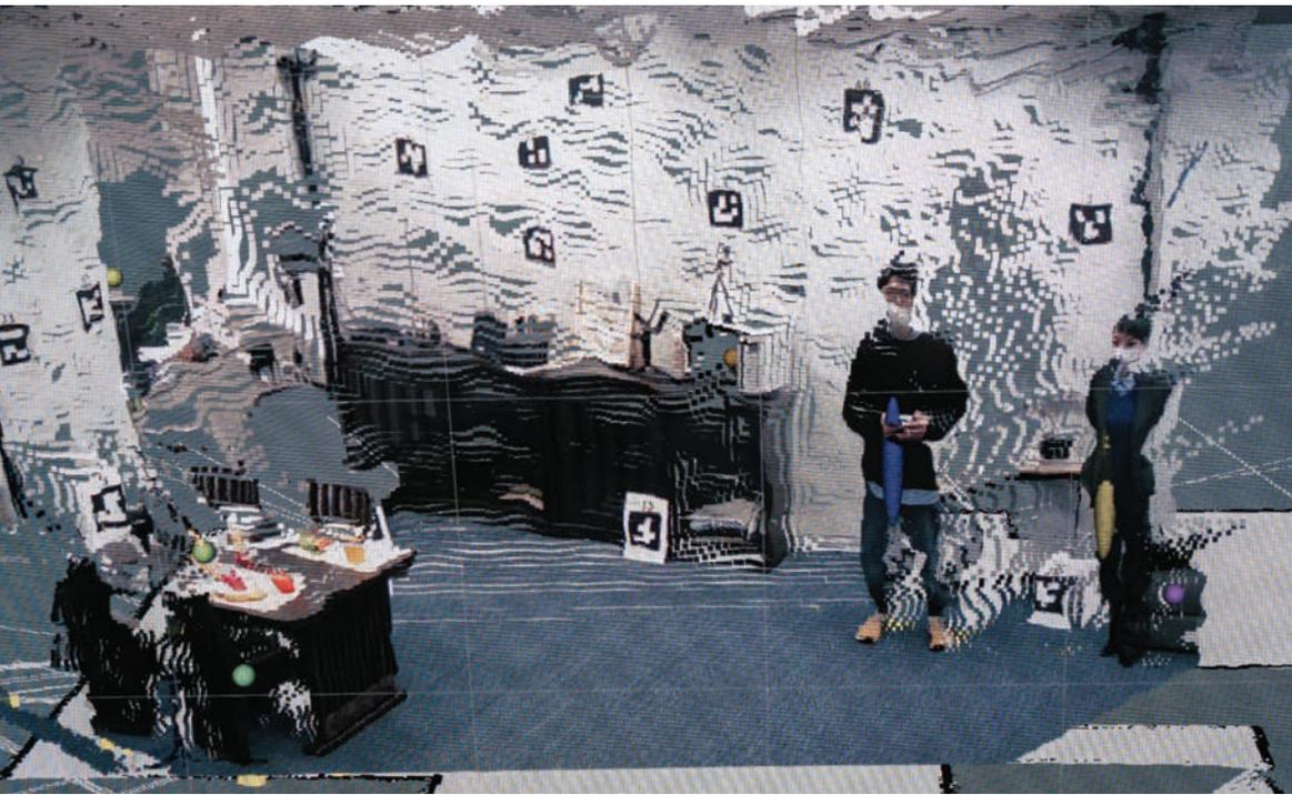
Task-oriented mobile robot, Butsukusa, autonomously patrols one of the GRP's rooms guided by a camera-and-laser system that helps it measure distance. It uses a deep-learning driven recognition module to identify objects, humans and the environment (above), as well as its location and speech. A combination of sensors that take in audio, visual and thermal information has been proposed to increase its ability to recognize people and their emotions.
