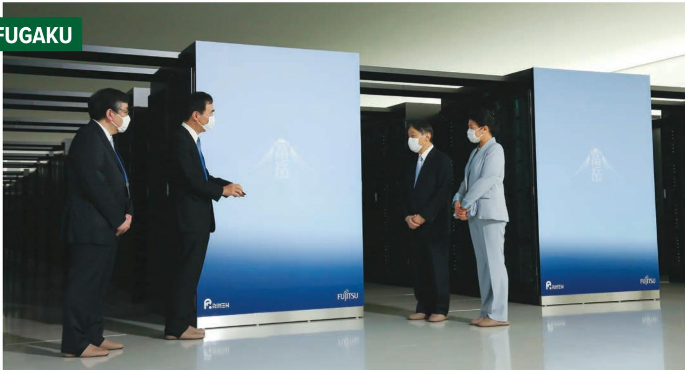
Supercomputer Fugaku is at the top of two rankings, the HPCG, which measures efficiency at processing relevant to real-world applications, and the Graph 500, focused on the ability to deal with data-intensive loads.
