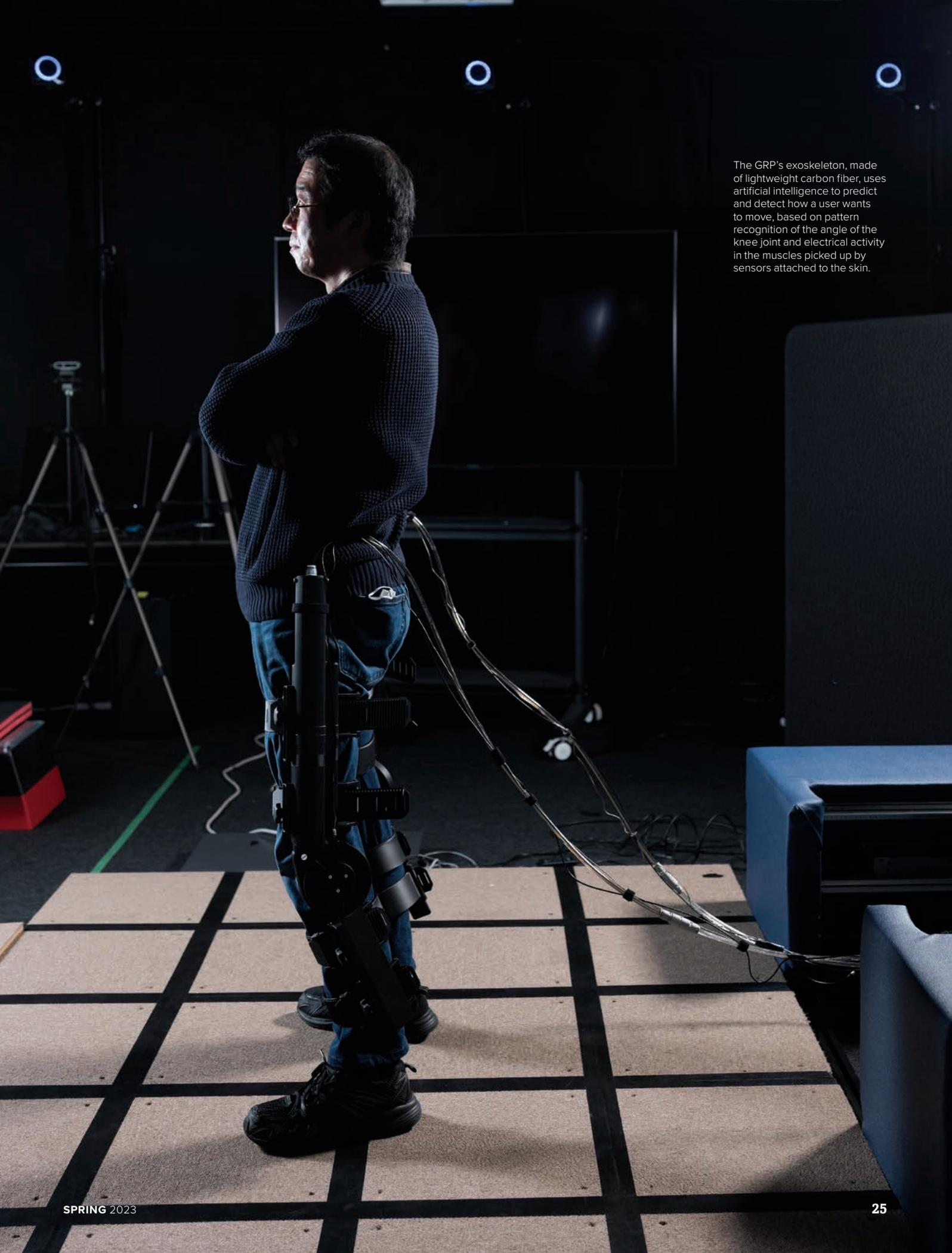
The GRP's exoskeleton, made of lightweight carbon fiber, uses artificial intelligence to predict and detect how a user wants to move, based on pattern recognition of the angle of the knee joint and electrical activity in the muscles picked up by sensors attached to the skin.
